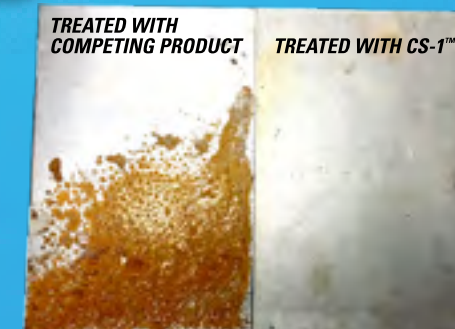
*Above 2 sheets treated and set outside at 30°-50° F for 5 days with a salt solution applied to surface each day.
